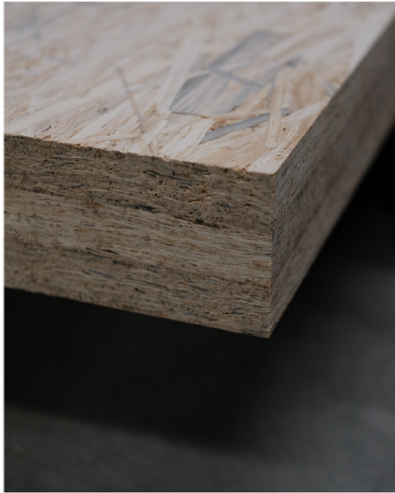
Three-layer UniStrand Element made from cross-laminated unidirectional single panels
